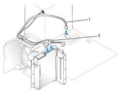
1 serial ATA data cable 2 power cable
