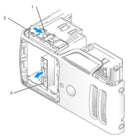
sliding plate lever sliding plate
